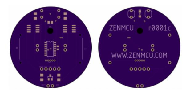
Architecturally this design is a Spanda card. While it is capable of operating on its own, and accepting 4th scripts via the HIF UART, the long term intent is for this to be controlled by another MCU; the Base, in Spanda terminology. However, I have taken to calling the r0001c the "Rykor", and the future controlling MCU as the "Kaldane". If you are not familiar with Edgar Rice Burroughs' Mars stories then that will mean nothing to you. If you are then that may make some sort of twisted sense.
